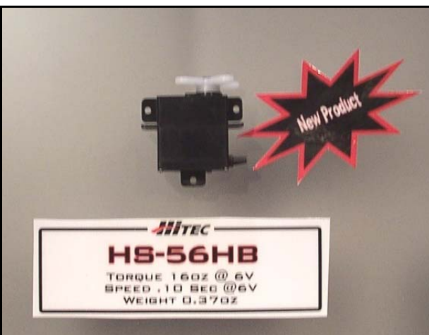
Like 'em small? Hitec debuted the HS-56HB, it's a variation on the popular HS55 servo. Differences? Karbonite gears and side tabs for easy mounting on the side of a depron/fanfold foam indoor-parkflyer model.
